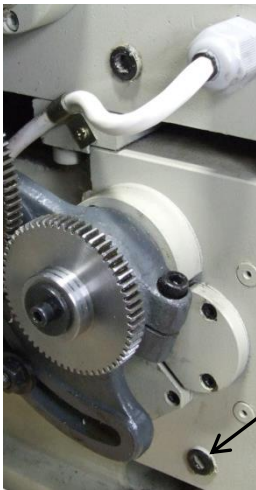
Gearbox Oil Drain
