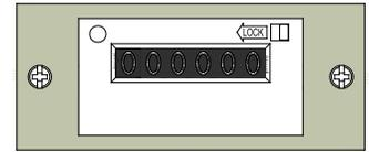
**POWER INDICATOR LIGHT** – When the disconnect switch is turned on the white light will be lit. Make sure machine is plugged into correct power source and that both E-Stop buttons have been reset.
