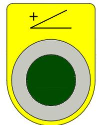
**RAKE ANGLE ADJUSTMENT ON - OFF SWITCH** – This selector switch must be “**ON**” in order for the rake increase / decrease pushbuttons to work.
