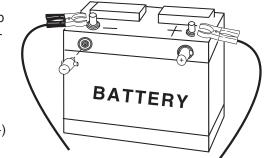
**NOTE:** Side mounted and threaded steel post batteries will require Lead Post Adapters. Using steel bolts and connecting clamps to threaded steel posts is not safe, and will inhibit accurate results.
