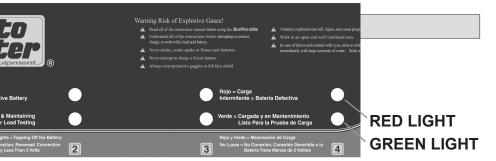
**Red & Green light = Finishing Full Charge.** "Ready for Load Test": The battery is at least 70% charged and ready to load test and return to service. Continued charging will take the battery to full charge.
