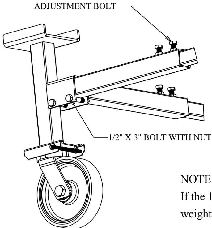
NOTE: The 3,000 lb weight rating pertains to the 8" polyurethane on cast-iron wheels shown. If the 10" solid rubber wheels are ordered, the weight rating is reduced to 2,000 lb with even weight distribution.
