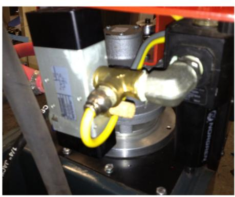
Maximum Operating Pressure70 Mpa10156 PsiMinimum Operating Pressure2 Mpa290 PsiHigh Flow Relief0.7 L/Min.19 G/MinLow Flow Relief2.4 L/Min.63 G/MinAir Motor Pressure.6 Mpa87 Psi
