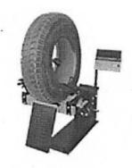
8. After finished maintenance work, please firstly move the up & down control valve to the downward direction, let the tire fall to the lowest, then move the up & down control valve to the direction of contraction, loosen the spreading hook and remove it from the tire core, then discharge the tire along the sloping board.
