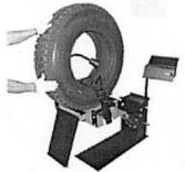
7. The work light fixed on the machine needs to be adjusted to a proper position, to illuminate the inside sufficiently and make the repair work easy.
