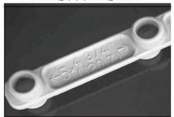
The **Wheel gauge** is the most useful tool to ever hit the wheel industry. It measures most wheels and brake hubs.
