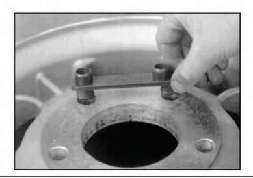
Wheels with conical seat lug holes (most wheels today) are easily measured using the two included conical adaptors. Using the adaptors allows the **Wheel gauge** to center on two adjacent lug holes. The measurement can be made from either the front or back of the wheel.
