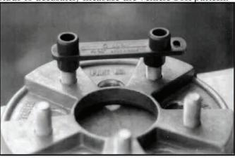
Aluminum wheels without conical seats are easy to measure by fitting the ends of the **Wheel gauge** completely into two adjacent lug holes.
