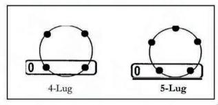
The **Wheel gauge** has holes molded into each gauge to fit over the studs of a vehicle. In some cases, the same bolt pattern is used by different vehicle manufacturers with a different stud size. This can cause the gauge to fit loose. Use caution when the gauge does not fit snug. It could be a different stud size but it might also mean you have selected the wrong gauge. We have molded in the stud size we feel is the most popular.
