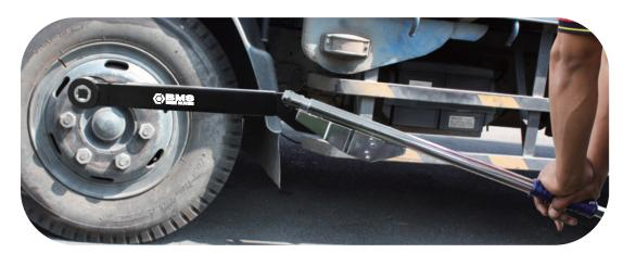
• Torque wrench mechanism will break-a-way when desired torque is met. Do not continue to apply pressure after desired torque is met.
