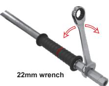
• To avoid inaccurate torque, do not fully remove the nut.
