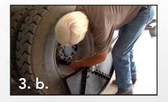
**3. b.** Install socket on the lug nut, slide **Torque Fin®** on the extension until it touches side wall of the tire.
