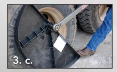
c. Use your foot to press Torque Fin<sup>®</sup> against the ground.
