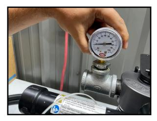
4. Install the output hose gauge. Index the gauge to face the operator while using the air inlet regulator and gauge assembly.
