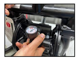
2. Install the Air Inlet Regulator and Gauge Assembly. Ensure to index the assembly so that the gauge and control are accessible to the technician.
