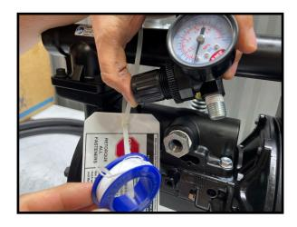
1. Locate the air inlet regulator and guage assembly. Pipe Tape or Pipe Compound is recommended to assist with indexing the assembly for eas of use.
