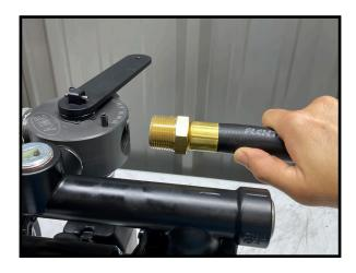
7. Locate the intake hose. This hose can be identified by the attached strainer.
