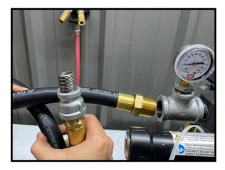
5. Locate the output hose. This can be recognized by the reducer present for mounting the Haltec 310 core ejector gun.
