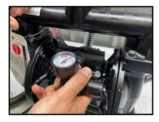
2. Install the Air Inlet Regulator and Gauge Assembly. Ensure to index the assembly so that the gauge and control are accessible to the technician.
