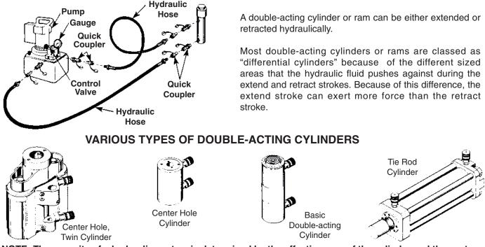
NOTE: The capacity of a hydraulic system is determined by the effective area of the cylinder and the system pressure.
