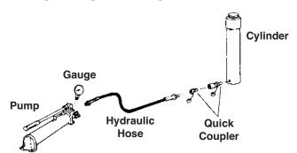
Since the single-acting cylinders have only one hose going to the cylinder, the cylinder can only apply force to extend (pull cylinders retract) its rod. The return stroke is accomplished by gravity or spring force.
