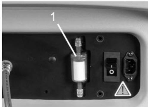
Fig. 34: Refrigerant identification unit
