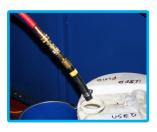
Connect any open end adapter to **red hose** and insert into appropriate disposal container. Pull diverter valve knob OUT.
