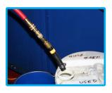
Connect any open end adapter to **red hose** and insert into appropriate disposal container. Pull diverter valve knob OUT.
