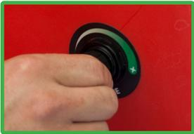
4. SLOWLY turn regulator clockwise until gauge pressure is a few lbs higher than the cooling system's rated pressure.
