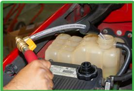
5. Insert open ended hose into reservoir to be filled.
