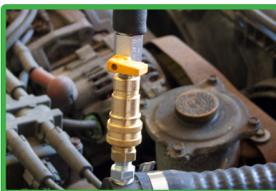
9. When the fluid runs clean, close the black hose ball valve and turn regulator counterclockwise to relieve pressure.
