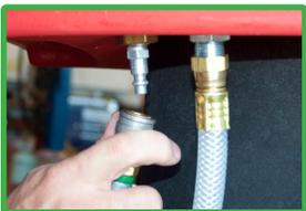
1. Connect air supply hose to air fitting on PSI-COOL machine.
