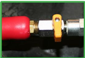
7. Close ball valve when fill is completed.
