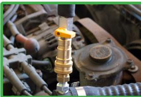
6. Allow machine to vacuum cooling system until no more fluid is flowing through the black service hose. When used coolant is no longer flowing, close ball valve on black service hose.
