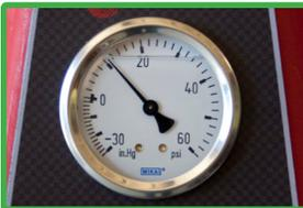
8. When gauge on control panel returns to 10 -12 PSI, open ball valve on black hose half way to allow fluid to be flushed through the vehicle's cooling system. Control the flow of coolant through the system using the ball valve on the black service hose.
