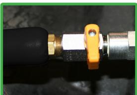
6. Close ball valve when drain is completed.
