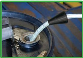
3. Open ball valve on black service hose and place in waste fluid container.
