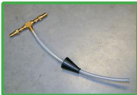
3. Connect both hoses to supplied rubber cone T-adaptor and open ball valve on black service hose only.
