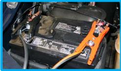
Connect battery cables to vehicle's battery.
