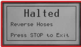
If the exchange stops and the display reads "Reverse Hoses", turn vehicle **off**, switch the red and black service hoses, restart vehicle, and press
