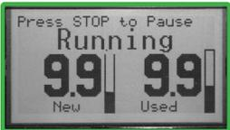
After cleaning for 10 minutes, the exchange begins. Once the exchange is complete the machine will beep and display "**Complete**".
