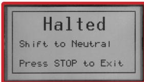
If the exchange stops and the display reads "Shift to Neutral", set the vehicle's parking brake, shift to Neutral, and press
