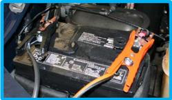
Connect battery cables to vehicle's battery.
