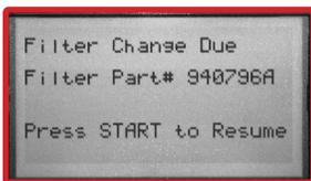
The machine will indicate when the canister filters need to be replaced. Remove service panel. Use a standard filter band clamp tool to unscrew old filters, and replace them with new filters. Make sure new filters are on tight.
