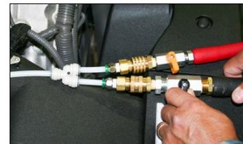
Fill the new fluid tank with the same amount of fluid that was extracted in the previous step.
