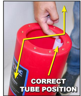
Line up nozzle with label as shown. Position nozzle gasket as shown and secure nozzle using four screws and four locknuts. Stand tank upright into bucket cradle and inspect that draw tube is positioned as shown.
