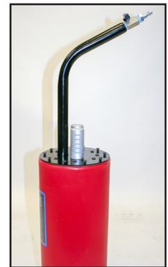
Align gasket and use an Allen wrench to tighten the screws securing the top assembly to the canister as shown. Use the label as a reference for positioning.
