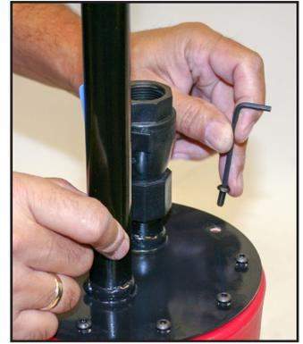
Install draw tube as shown with 1" overlap, and tighten hose clamp. Align gasket and use an 1/8 Allen wrench to tighten the screws securing the bottom assembly to the bottom of the canister. Be sure drain valve is opposite the label as shown.
