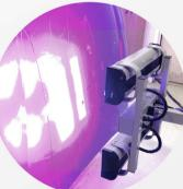
UV curing is the process by which ultraviolet light is used to initiate a photochemical reaction that generates a crosslinked network of polymers. UV curing is adaptable to printing, coating, decorating, stereolithography, and in the assembly of a variety of products and materials.
