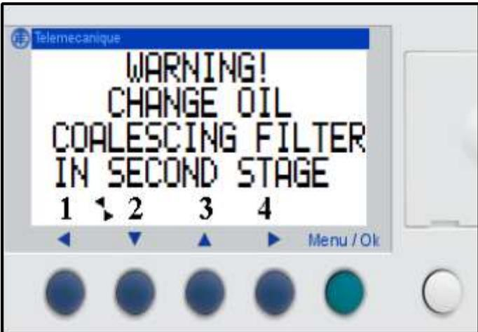
1. Change oil coalescing elements prior to resetting your PLC. For instructions on how to change element, see Maintenance Instructions for coalescing elements on page 4.
